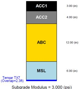
Subgrade Modulus = 3,000 (psi) Structural Number = 4.540 Calculated Traffic (ESALs) = 615,000
