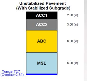
Subgrade Modulus = 3,000 (psi) Structural Number = 2.880 Calculated Traffic (ESALs) = 750,000
